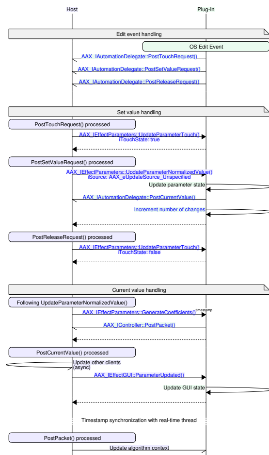
Figure 12.8 High-level sequence of interface calls and events for a parameter update following a user-generated edit
